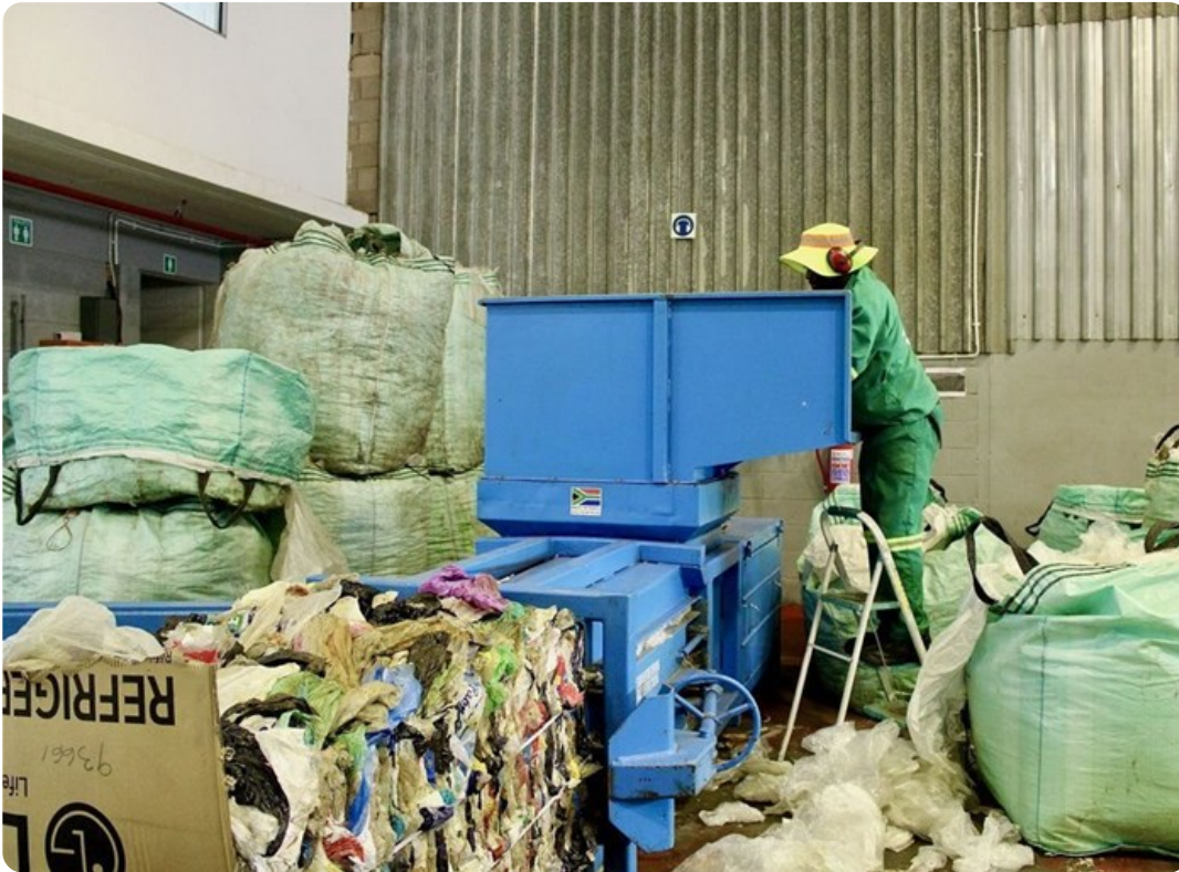
Recyclable items collected and sorted at the African Reclaimers Organisation's sorting centre are compressed using a baler machine before being sold to buy-back centres. Photo: Masego Mafata / GroundUp
