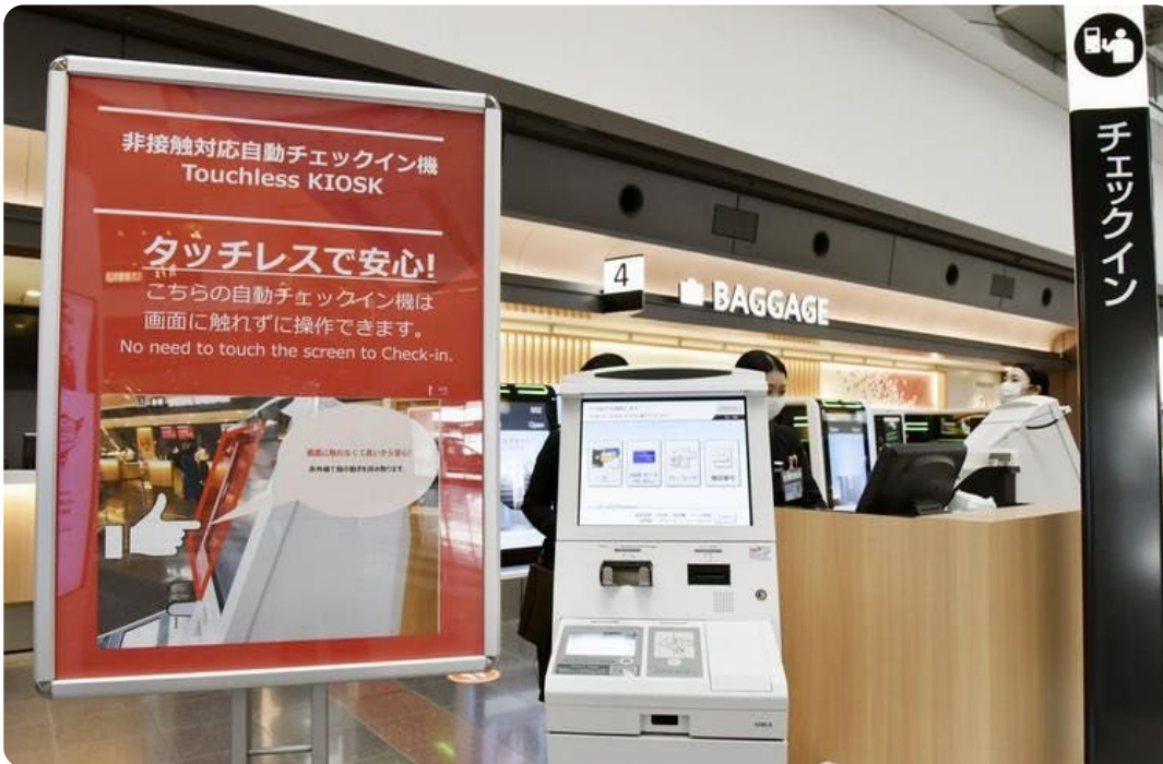
New self-service check-in machines introduced by Japan Airlines at Tokyo's Haneda airport enable passengers to complete the procedure without touching the screen. Kyodo/AP
