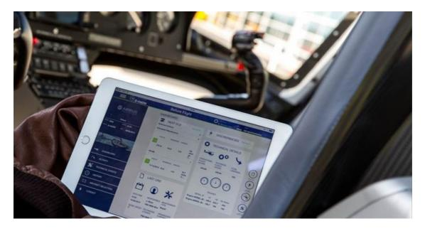
Fleetkeeper provides a helicopter's airworthiness status to the pilots and records technical events during aircraft operation and any additional maintenance or repairs performed in-between scheduled base maintenance visits.
