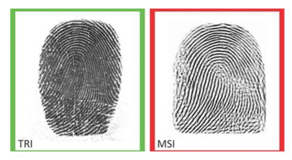
The picture on the left was obtained using a conventional TRI fingerprint scanner. Any experienced fingerprint expert will agree with me that this is a good quality print. The fingerprint ridges, core and delta are clearly visible. The contrast is obvious and even the sweat pores are noticeable. Most fingerprint identification systems will be able to easily assign the matching points with a high level of accuracy.
