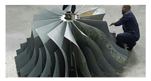
"The use of composites in these systems allows us to re-engineer the vapour compressor and blades that can withstand the highly loaded application where each blade experiences loads of up to 70 tonnes."
