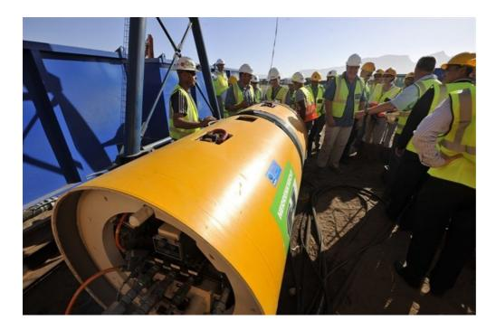
The machine has been used in more than 1,000 projects around the world. It is controlled with a laser navigation system that allows for precise positioning, has a built-in crusher that can reduce boulders to smaller pieces, and offers extra safety in less stable geological conditions (which is useful for tunnelling operations in the sandy Cape Flats soil).
