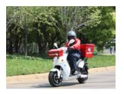
"Both scooters performed faultlessly during the whole tour over a distance of 520 kilometres," says Johan Prins, manager of the Post Office's fleet. "With one overnight battery charge the scooters can travel more than 80 kilometres with a top speed of 80 kilometres per hour."
