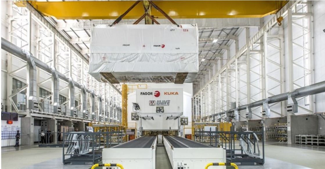
The press bed, weighing 120 tons, was lifted 8m over the existing press line.
