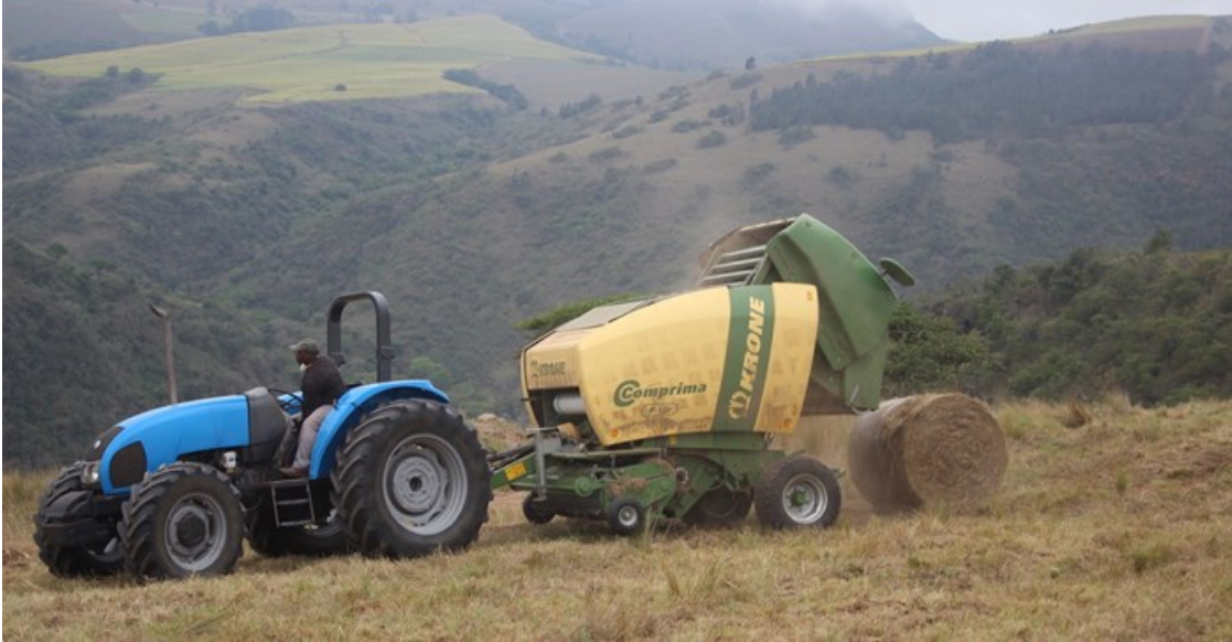
A baling machine collects loose grass and turns it into bales on a farm in Mid-Illovo to be transported to farmers in need in the Eastern Cape
