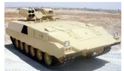
Denel's Ingwe missiles are fitted to a Jordanian Temsah APC. Image: Defence
