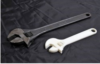
Fully functional shifting spanner was the first item print. Image: www.quickpic.co.za
