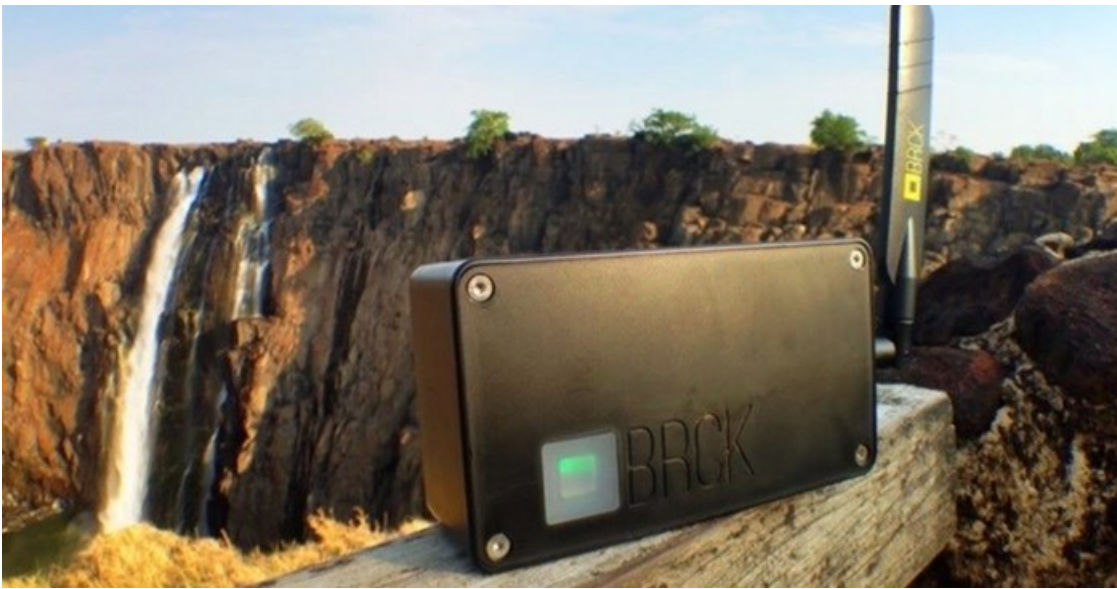
The BRCK: a rugged, self-powered, mobile Wi-Fi device which connects people and things to the internet in areas of the world with poor infrastructure.
