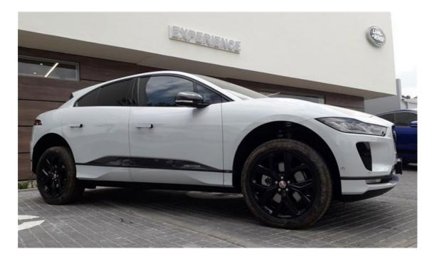
What's highly noticeable is the flush door handles, which keeps the clean and modern look, and I've been told that this contributes to the superb aerodynamics. What's impressive, is that the handles only appear at the push of a button or when the handles are touched.
