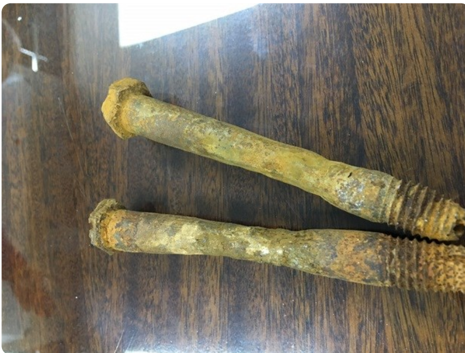
Steel screws show corrosion
