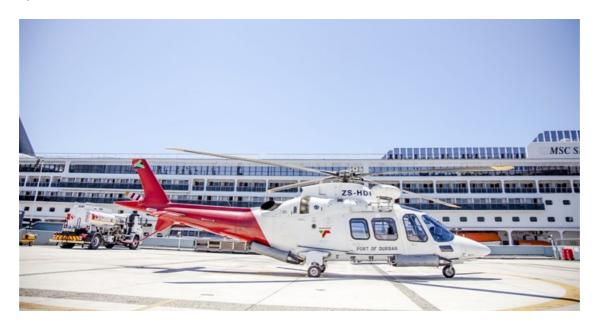
The AW109 series includes a twin engine and a harbour pilot kit that features a hoist to enable this unique operation.
