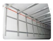
The lightweight - yet highly durable - double stacking system can be used in both refrigerated and dry freight trailers, with the entire system adding just 640kg in weight to a vehicle.
