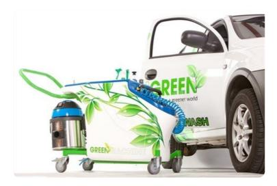
The machine dispenses an environmentally friendly wax through a pressurised system. The wax suspends dirt away from vehicle's surface and is wiped away with a special microfibre cloth, which is regularly rinsed. The wax, cloths, environmentally friendly wheel, mag and window cleaner and an industrial vacuum cleaner are all contained in a compact push-trolley design that is small enough to fit between parked vehicles.
