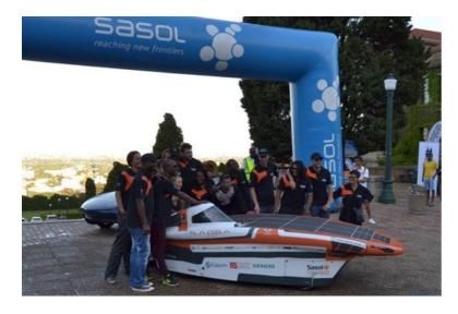
The solar cells, used in the array of Ilanga II are commercial cells imported from Germany for space grade applications. The car has Gallium Arsenide (GaAs) solar panels, which are the same type of panels as those used on the Mars Rovers.
