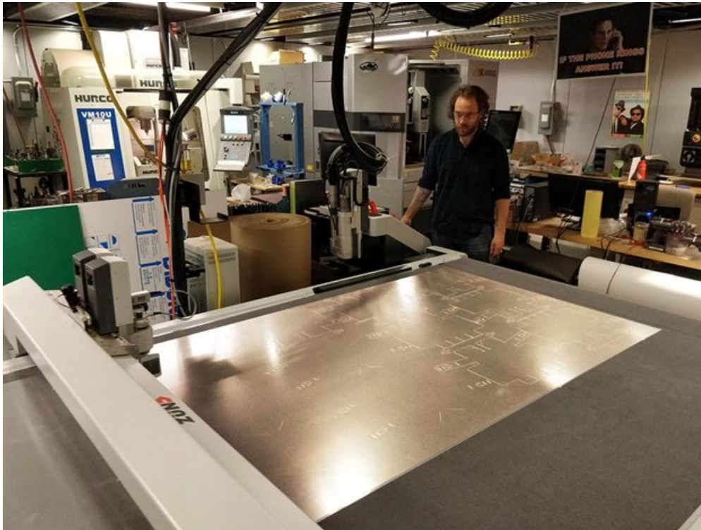
Graduate student Zach Fredin operates the Zund large-format cutter in MIT's Center for Bit and Atoms. The machine was used to make prototypes of the face shield. Image © Center for Bits and Atoms
