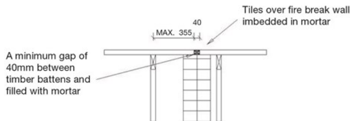
TYPICAL FIRE BREAK BETWEEN TWO FLATS OR TOWN HOUSE UNITS
